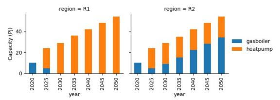
We can see that R2 quickly reaches its capacity limit for heatpump, and additional investment in gasboiler needed to meet the residential heating demand.
