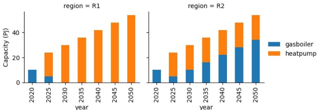
We can see that R2 quickly reaches its capacity limit for heatpump, and additional investment in gasboiler needed to meet the residential heating demand.
