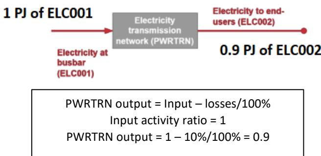
Add the values of the Output Activity Ratio in “Data entry” for the “Output Activity Ratio” parameter, as calculated above (and summarised in the figure below for your convenience).
