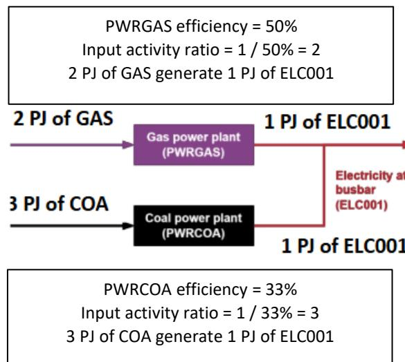
**NOTE:** Conversion efficiencies are determined by the relative magnitudes of the input and output activity ratios.
