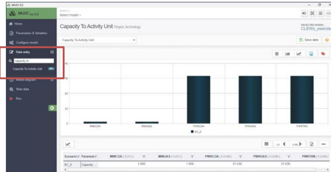
**NOTE:** 31.536 corresponds to the energy, expressed in PJ, which can be generated or transferred by an electricity system technology with 1GW capacity and 100% efficiency in one year.
