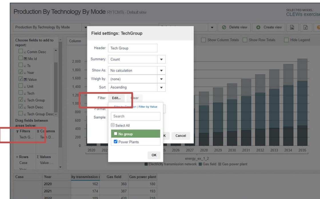
The results for “Production By Technology By Mode”, displayed in the figure for the group “Power Plants”, correspond to the generation by power plants over the modelling period.
