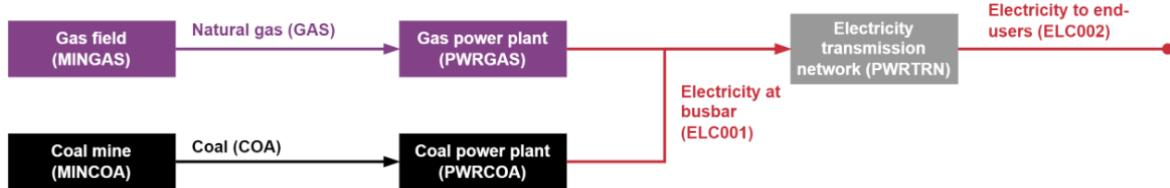
Example: COA is an output of technology MINCOA and an input to technology PWRCOA
