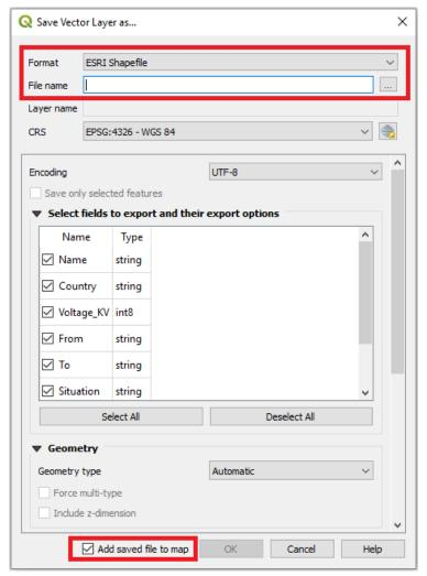
3. Name your layer "transmission\_lines\_Benin" and navigate to the folder named Transmission\_Lines that you have received. Click "OK" (make sure that "Add saved file to map" is checked). Now you can remove the temporary file named "Clipped", by right-clicking and selecting Remove Layer.
