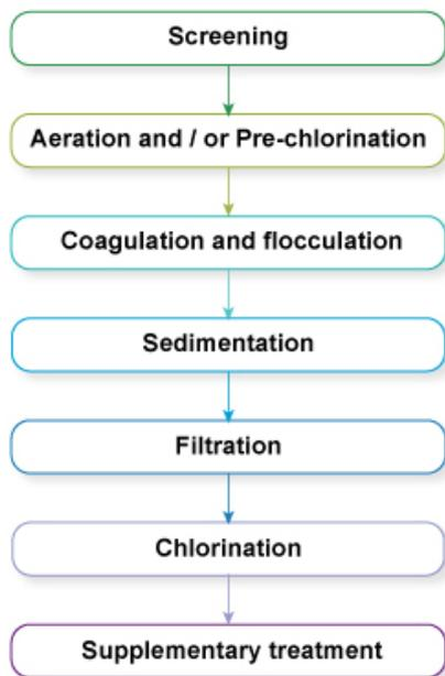
*Figure 5.2 The seven steps often used in the large-scale treatment of water.*
