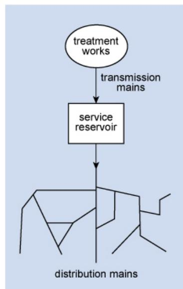
Figure 1.10 A simple water distribution network.
