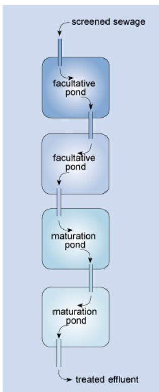
Figure 11.7 Layout of a waste stabilisation pond system for treating domestic wastewater.
