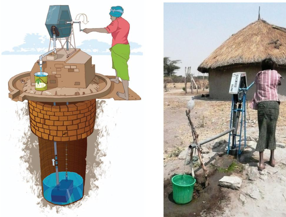
Figure 3.7 Examples of rope pumps.
