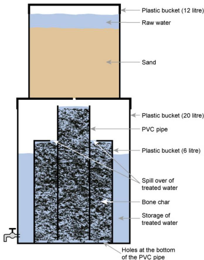
Figure 5.8 The Nakuru method for defluoridation using plastic buckets and piping.
