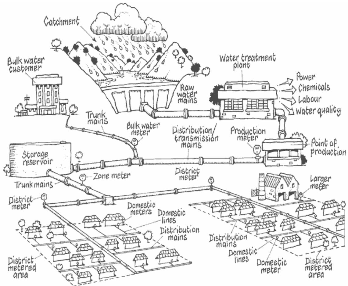
Figure 8.3(a) A water supply system.
