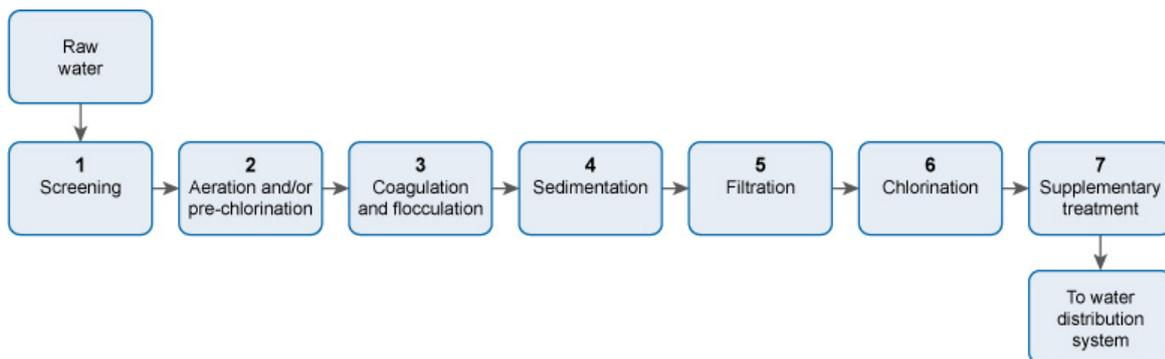
Figure 5.9 The seven-stage process of water treatment.
