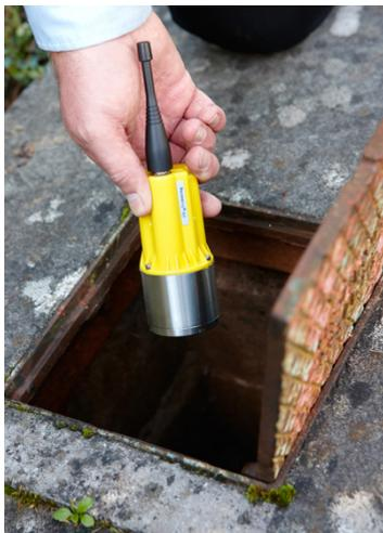
*Figure 7.6 An acoustic logger to detect leaks through a change in noise level in the water pipe.*
