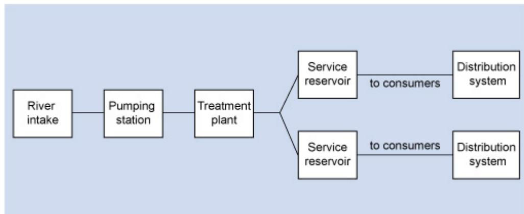
Figure 8.3(b) The elements of a water supply system.
