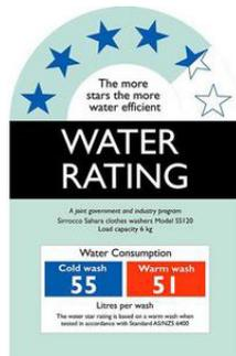
*Figure 11.3 Label indicating water use by the appliance.*
