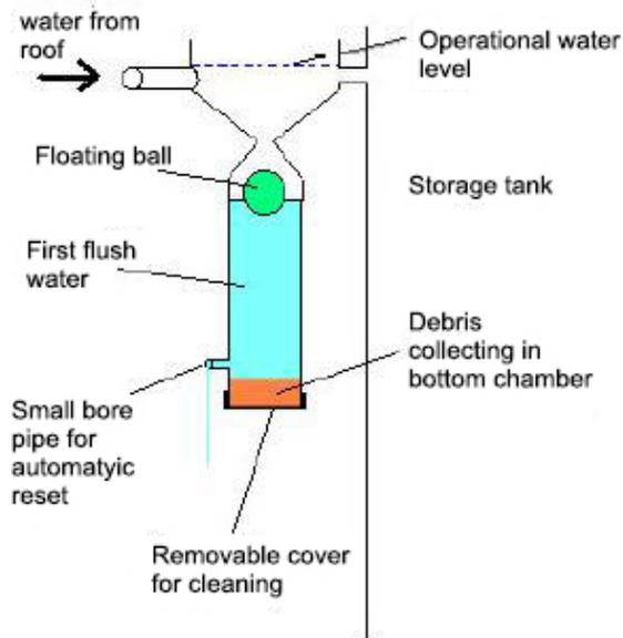
Figure 11.5 The floating ball first flush system.
