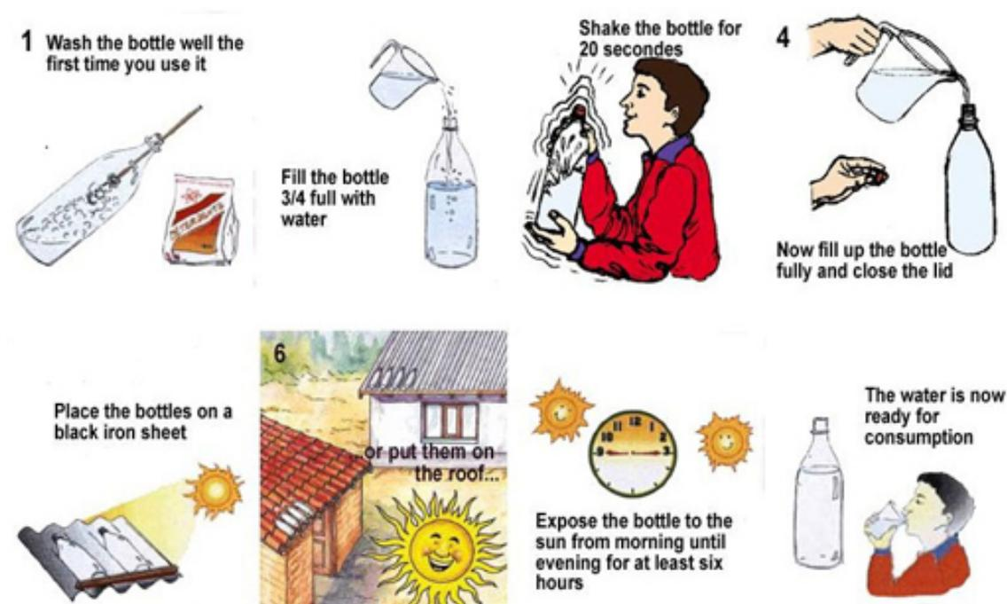
Figure 10.9 The procedure for solar disinfection of water (SODIS).
