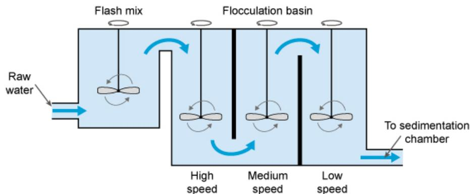
Figure 5.5 The coagulation–flocculation process.
