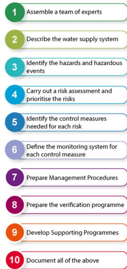
*Figure 8.1 The steps in a Water Safety Plan.*
