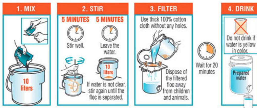
Figure 10.13 How to use P&G Purifier of Water.
