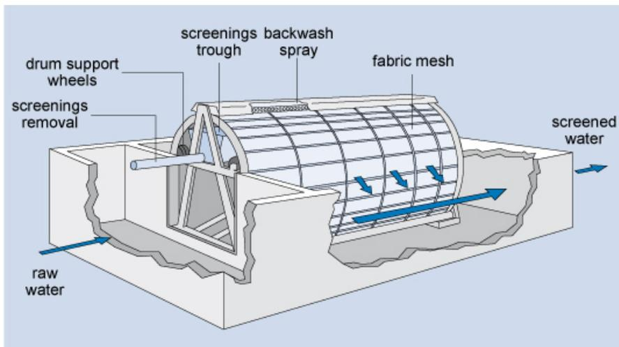
Figure 5.4 Diagram of a microstrainer.
