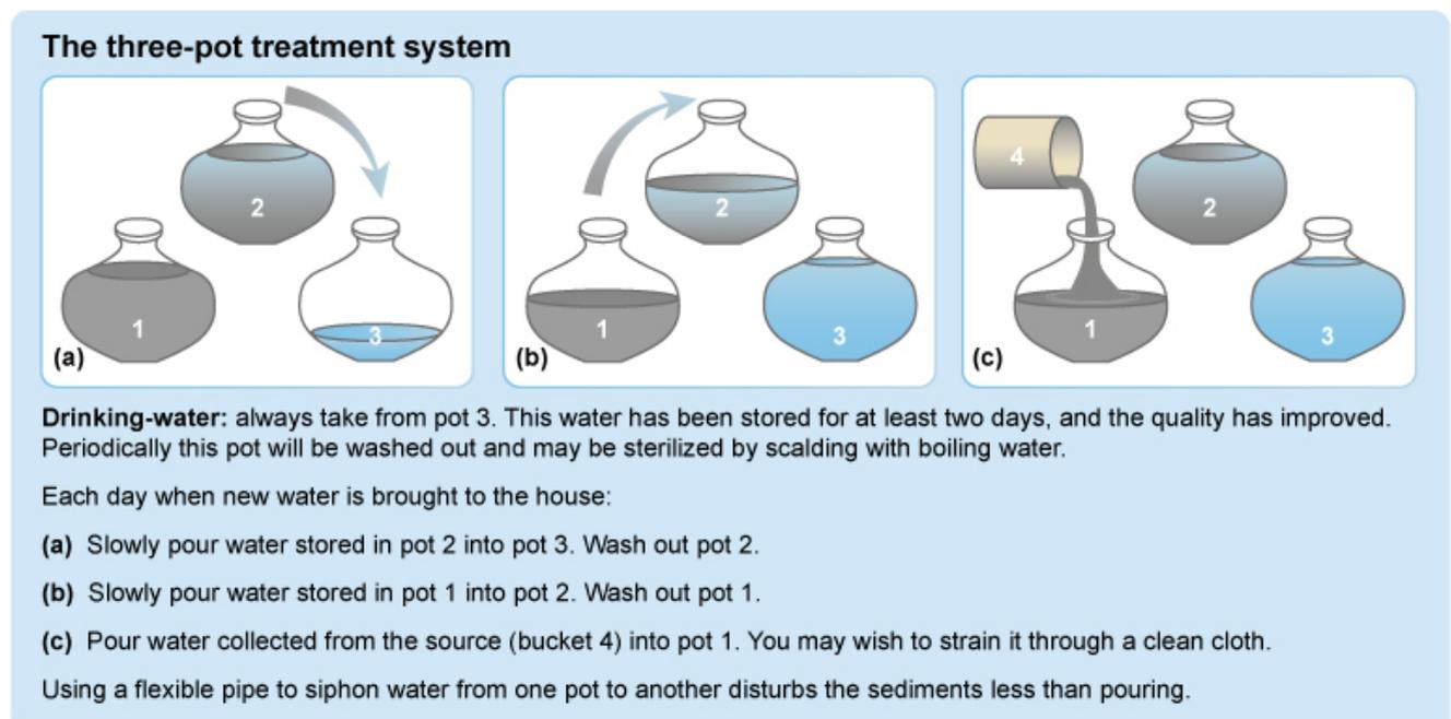
Figure 10.4 The three-pot water treatment system (IFRCRC, 2008).
