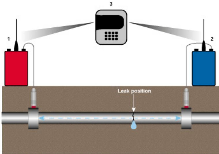
*Figure 7.5 A noise correlator system to pinpoint the location of a leak.*
