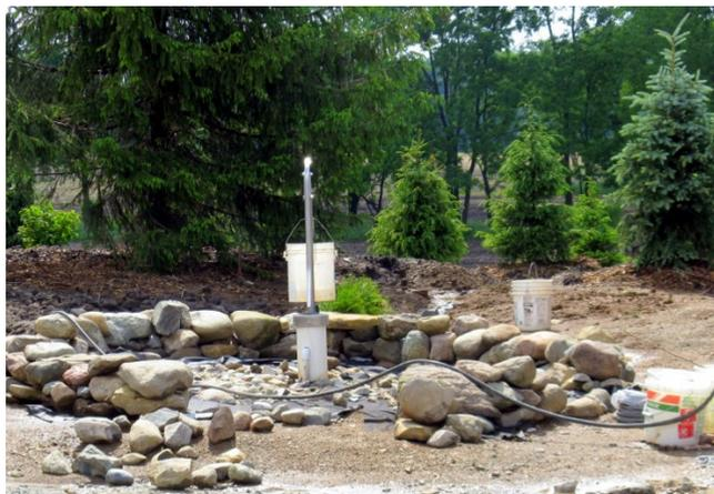
Figure 3.16 Hand pump over a well.
