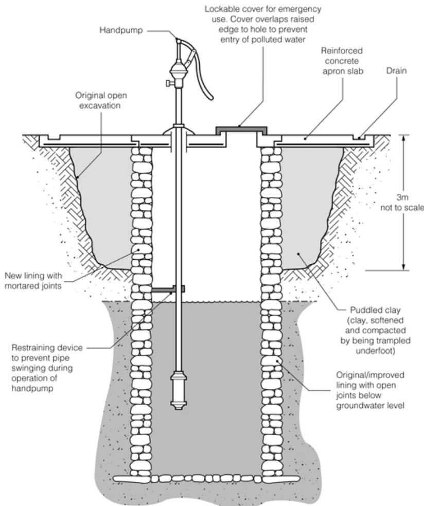
Figure 3.4 Diagram of a hand-dug well.
