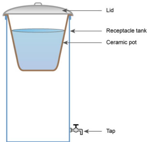
Figure 10.7 Ceramic pot method of water filtration.
