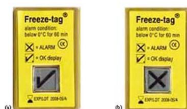
Figure 6.9 Freeze-tags showing: (a) ‘good status’ display; (b) ‘alarm status’ display. (Photo: WHO)
