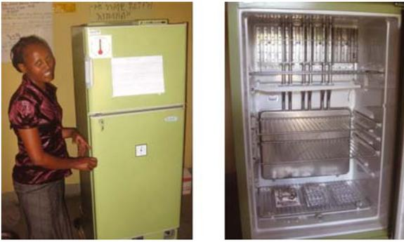
Figure 6.2 A Health Extension Worker with a kerosene-powered refrigerator in a rural Health Post in SNNPR, Ethiopia. This refrigerator has a freezer compartment on top, and plenty of space for the vaccines, diluents and other supplies that must be kept cold. (Photos: Janet Haresnape)
