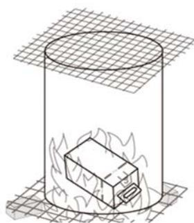
Figure 7.4 Burning a safety box in a metallic drum. (Source: WHO, 2004, *Immunization in Practice*, Module 4, *Ensuring safe injections*, Figure 4I, p.17)
