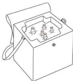
Figure 6.6 Foam pad with vaccine vials inserted. (Source: WHO, 2004, as in Figure 6.1, p.8)
