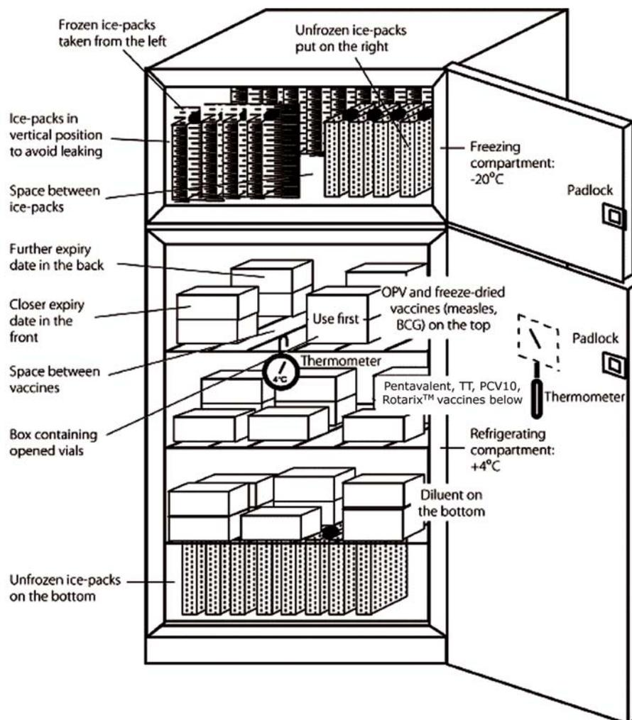
Figure 6.12 Front-loading refrigerator with separate freezing compartment on top. (Source: WHO, 2004, as Figure 6.1, p.18)
