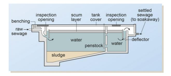
Figure 4.6 Cross-sectional diagram of a septic tank.
