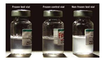
Figure 6.10 Three vials of liquid freeze-sensitive vaccine viewed with the light behind them: (left) frozen test vial in which a sediment has settled to the bottom of the vial after vigorous shaking; (centre) frozen control vial in which the sedimentation rate can be compared with the rate in a suspected frozen test vial; (right) non-frozen test vial showing the uniformly cloudy appearance of a vaccine that has not been damaged by freezing. (Photo: WHO)
