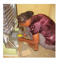
Figure 6.15 A Health Extension Worker checks the kerosene tank of a kerosene refrigerator. (Photo: Janet Haresnape)
