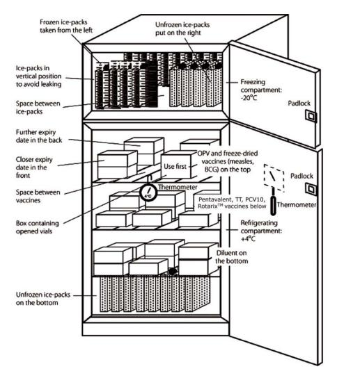
Figure 6.12 Front-loading refrigerator with separate freezing compartment on top. (Source: WHO, 2004, as Figure 6.1, p.18)
