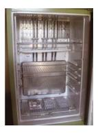
Figure 6.2 A Health Extension Worker with a kerosene-powered refrigerator in a rural Health Post in SNNPR, Ethiopia. This refrigerator has a freezer compartment on top, and plenty of space for the vaccines, diluents and other supplies that must be kept cold. (Photos: Janet Haresnape)
