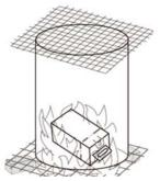
Figure 7.4 Burning a safety box in a metallic drum. (Source: WHO, 2004, *Immunization in Practice*, Module 4, *Ensuring safe injections*, Figure 4I, p.17)
