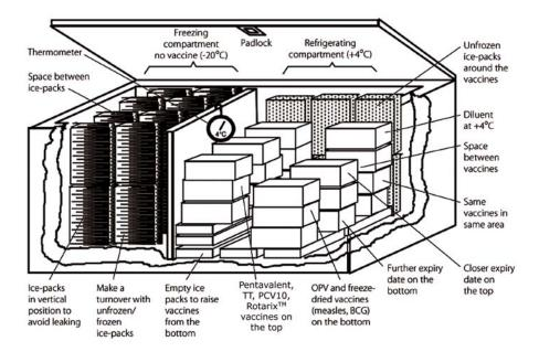
Figure 6.13 Storing vaccines in an ice-lined refrigerator. (Source: WHO, 2004, as in Figure 6.1, p.19).
