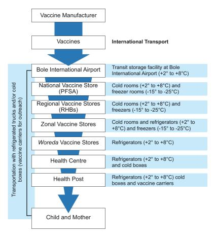
Figure 6.1 The cold chain. (Adapted from: WHO, 2004, *Immunization in Practice*, Module 3, *The Cold Chain*, Figure 3A, p.2)
