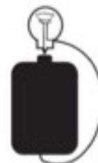
This model is specially designed so that you can demonstrate the arrangement of the inner parts of the bulb. What happens inside a light bulb will always be a strange mystery to students unless they have thought about what might be the case, and then had the chance to find out. It is possible to use a hack-saw blade to carefully cut open the metal case of an old screw-in bulb. Then the arrangement and direction of the wires is clear.
