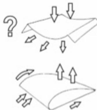
A third thing to try is to fold a sheet of A4 paper slightly off-centre, and then to glue down the two ends to form a model of the wing of a plane or a bird. Blow straight against the front edge and see what happens. The paper model lifts up. Why?
