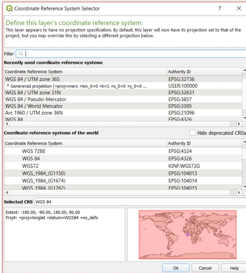
In the filter field start typing the name of the coordinate system you want to use (“**WGS 84/UTM zone 31N**”):
