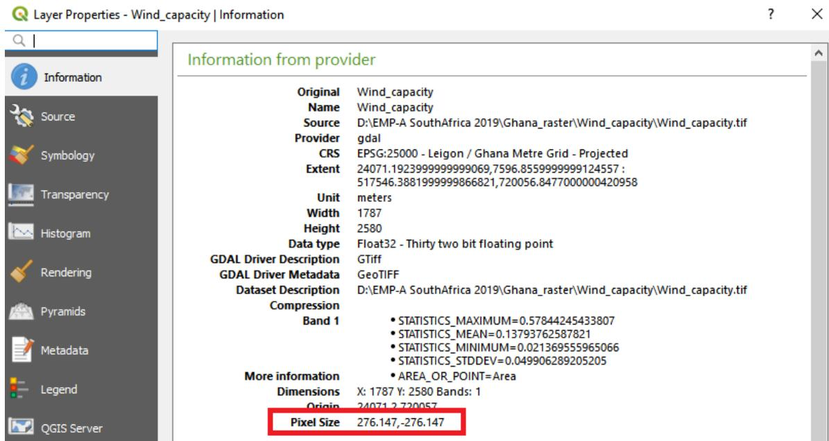
As the unit of the coordinate system is in metres, this is equivalent to a spatial resolution of 276 m<sup>2</sup>. We want the spatial resolution to be 1 km, in other words, we want the wind capacity raster to have a cell size larger than the one we have now. This can be done by resampling the map, using a tool named **r.resamp.stats**.
