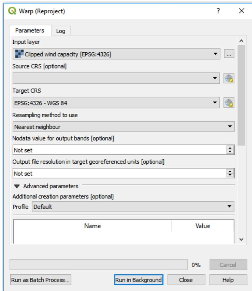
3. You do not need to specify the current projection system used for the raster, so the second field ("Source CRS [optional]") can be left empty.
