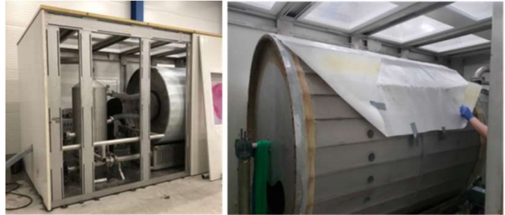
S3 filterdryer demonstration unit as produced by Salten Havbrukspark/LS Optics AB. Right frame show the details of the filter during change of filter cloth. See https://youtu.be/UD7csMyUVtQ for operation.
