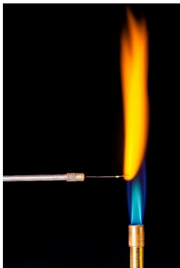
Figure 5. Flame test for sodium ions.
