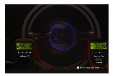
**Figure 4** The fine beam tube from the application in operation with a lilac circular beam shown.
