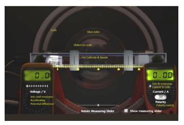
**Figure 3** The fine beam tube from the application, with the beam turned off and measuring slider displayed.
