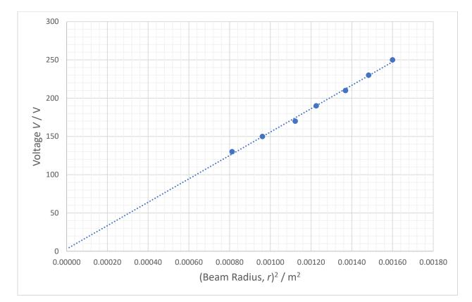
Graph showing Voltage against (Beam Radius)<sup>2</sup> for the Fine Beam Tube, current fixed at 1.52 A
