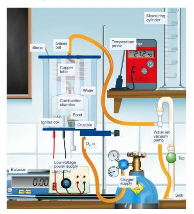
Figure 9. Simple food calorimeter
