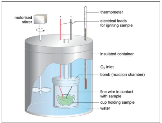
Figure 10. A bomb calorimeter
